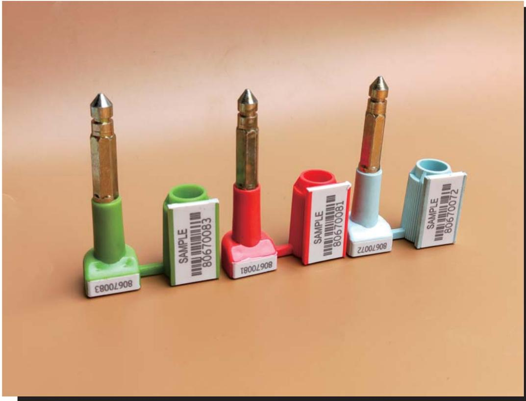
The bolt seals complies with ISO17712, To avoid opening it with rotating method. The new structure has metal antispin design. if so, It only can be opened by cutting or loading. The tensile strength is more than 1850kgs.
